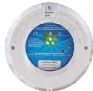
Pulsing LEDs confirm positive ground condition
